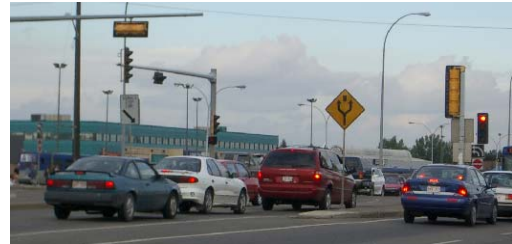
Eastbound left-turn vehicles: Note that a larger vehicle, such as the red minivan, may obstruct the visibility of the one left-turn signal from smaller vehicles behind it.
